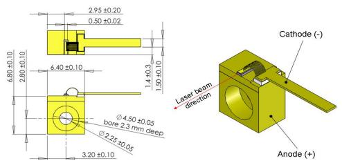
The C-mount is an ideal component for quick prototyping and laboratory setups. However, the maximum output power is typically limited by the inherently sub-optimal heat dissipation properties of the C-mount itself. Please contact us to discuss the best package option for your application.
