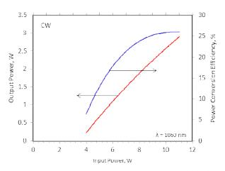
Note: The consumed power includes the power of the cooling system. The measurement was performed at typical ambient temperature (20°C). The consumed power varies depending on ambient temperature.
