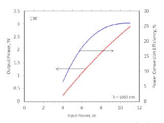
Note: The consumed power includes the power of the cooling system. The measurement was performed at typical ambient temperature (20°C). The consumed power can vary depending on actual temperature conditions.
